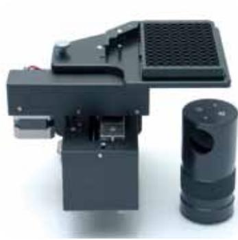
HTS/Raman accessory for high throughput FT-Raman spectroscopy.
