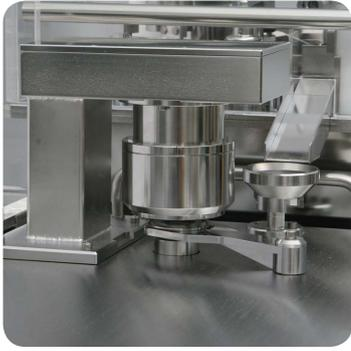
Automatic and accurate tablet positioning under the NIR transmission detector head for highest reproducibility.
