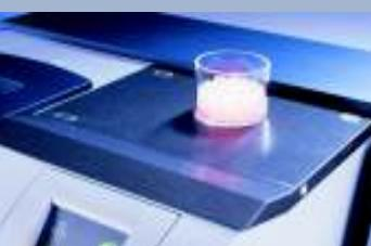
The integrating sphere of the MPA spectrometer
