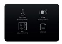
OPUS-TOUCH and its predefined workflows enable fast and unambiguous verification of raw materials. It provides accessibility for FTIR beginners and full instrument control for experts.
