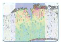
Combined with a FPA detector (focal plane array) the HYPERION offers FTIR imaging to answer complex analytical questions on material composition and content distribution.
