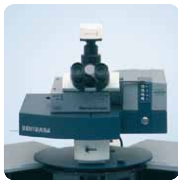
The "hybrid" platform enables the use of both Fourier transform and dispersive based Raman systems on a single microscope.
